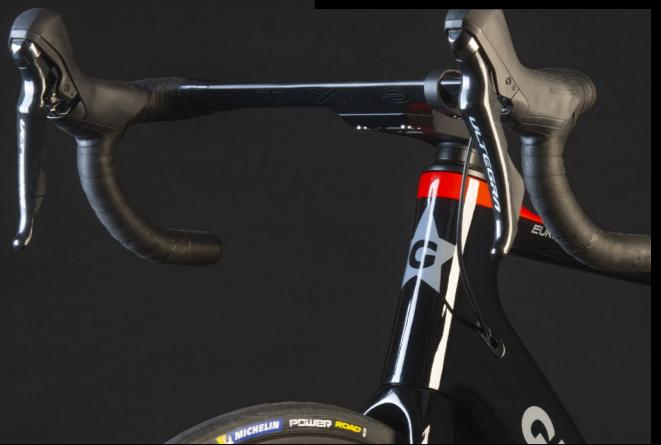
Aerodynamic, safety and elegance of the bike are ensured by its special ALL IN handlebar: we studied a internal cable routing system which eliminates any eventual issue in the steering zone.
