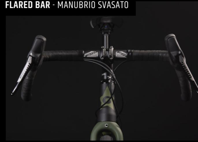
A flared handlebar is equipped on Greto. Its particular shape, now identifying the gravel segment, facilitates the control of the bike on gravel or dirt roads. A choice oriented towards comfort and safety, which also allows the mounting of a handlebar bag.
