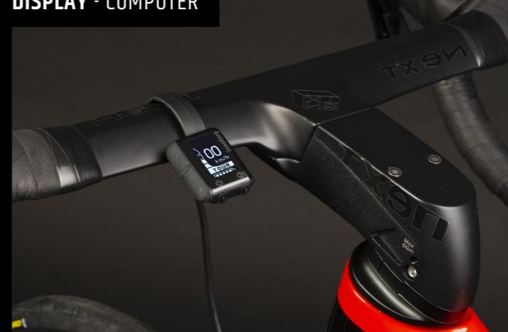
The Innotorq display equipped on the handlebar allows you to check speed, pedal assistance level, battery charge level and BLE connectivity.
