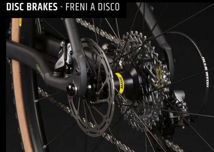
The disc brakes give an effective braking experience. In gravel cycling, where you might have to deal with muddy and wet conditions, this is crucial. The hydraulic cables are fully integrated within the frame: the result is a safe and aesthetically clean bike.
