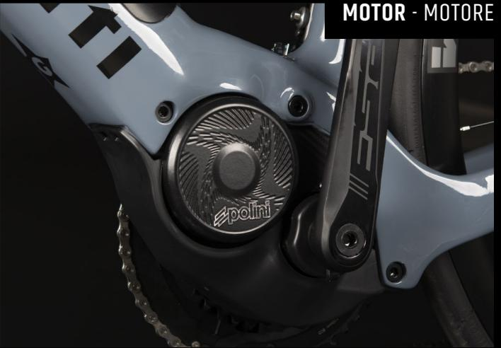
Navir I.ON's electric assistance is powered by a powerful 250 watt Italian motor, with a maximum torque of 70 N / m. Polini E-P3 boasts a unique design, compact size and lower weight than the e-bike motors available on the market today. Polini E-P3 offers 5 different levels of assistance. In addition, the 6 km / h walk assistance mode is available, which can be activated via the display and useful if you need to push your Navir I.ON by hand.
