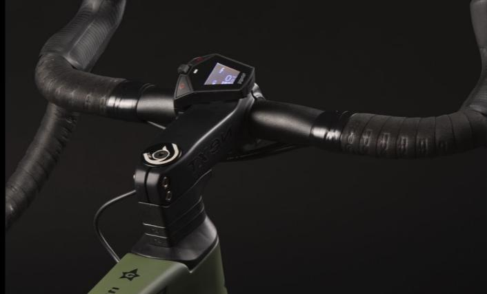
The DOT Matrix display mounted on the Brera I.ON handlebar allows you to control, via the integrated Joystick, the functions of your e-bike. The informations remain readable in all lighting conditions thanks to the ambient light sensor. Keep an eye on the level of support, battery charge status, speed, pedaling power and motor power. You can also control the lighting system and activate the assisted walking mode.
