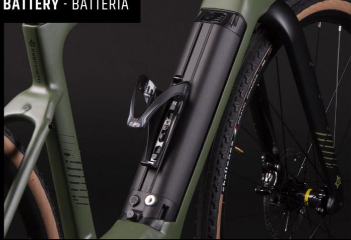
Brera I.ON is equipped with a 500 Wh lithium-ion battery, which will give you a range of assistance up to 220 km. Its special design allows it to be integrated within the frame. The battery support, designed to reduce the visual impact, is made of drawn aluminum. It also integrates perfectly with the engine mount, hiding the control cables inside.
