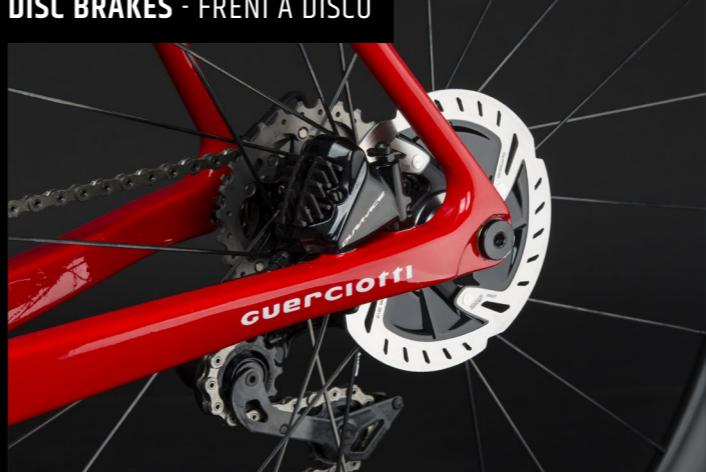
The disc brakes allow a perfectly safe braking experience. The hydraulic cables are fully integrated within the frameset, this gives the bike a maximum aerodynamic performance.
