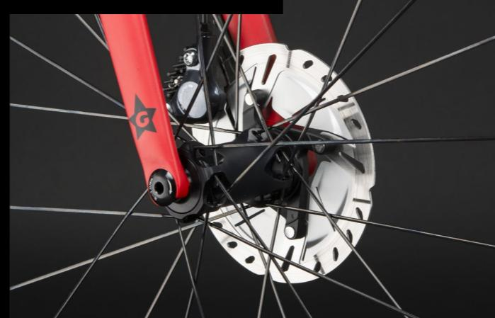
The disc brakes allow a perfectly safe braking experience. The hydraulic cables are fully integrated within the frameset, this gives the bike a maximum aerodynamic performance.
