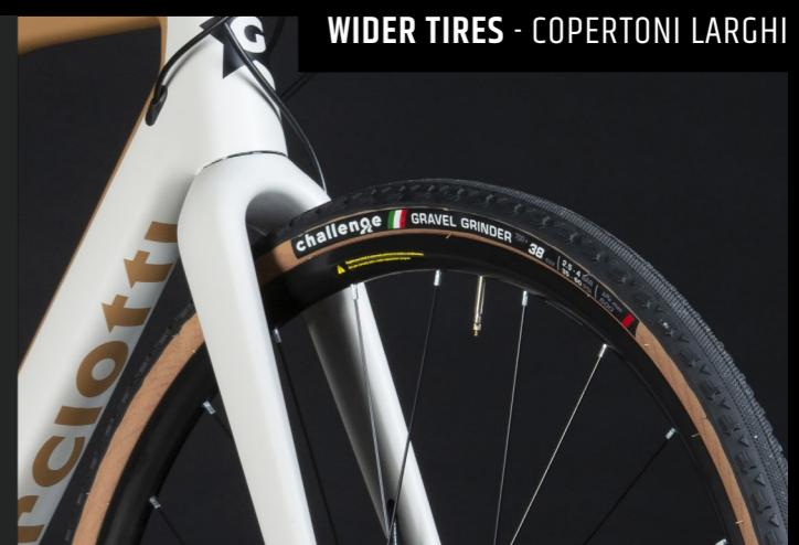
The fork design allows the mounting of wide rims with "oversize" tires (up to 42 mm). This solution, derived from cyclocross, provides stability to the bicycle. Inflated to lower pressures than classic racing tubulars, these tubeless tires stay glued to the road. Reliability, comfort and safety for your gravel rides.
