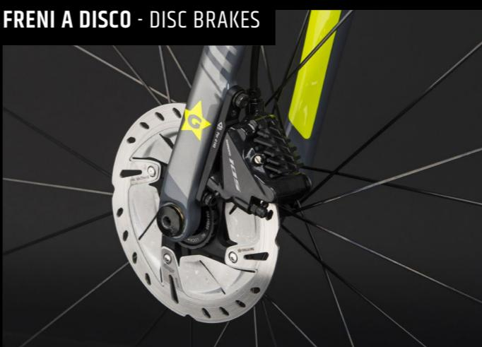
The disc brakes allow a perfectly safe braking experience. The design of fork and frame was updated to meet the standard disc brakes requirements.
