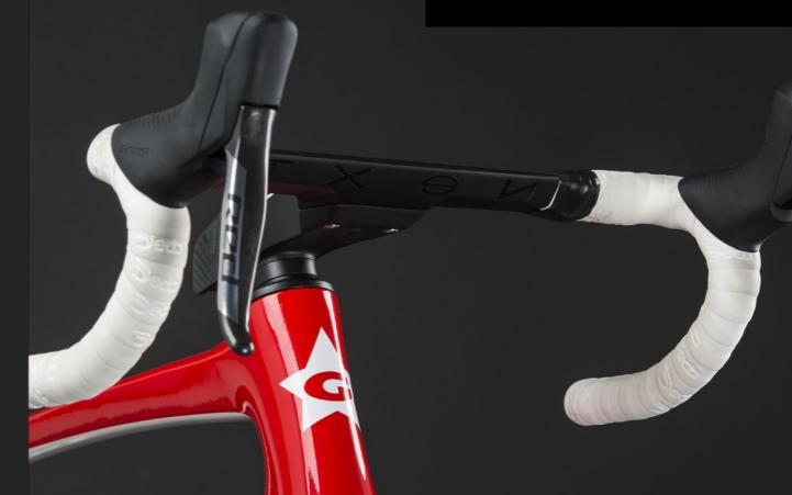
Aerodynamic, safety and elegance of the bike are ensured by its special ALL IN handlebar: we studied a internal cable routing system which eliminates any eventual issue in the steering zone.
