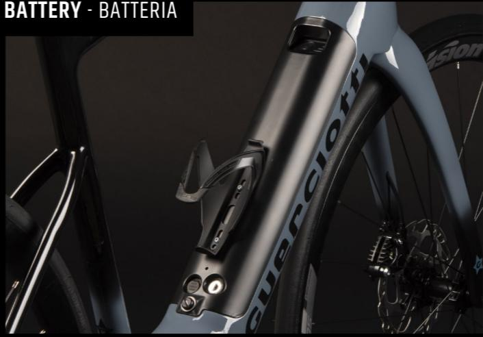
Navir I.ON is equipped with a 500 Wh lithium-ion battery, which will give you a range of assistance up to 220 km. Its special design allows it to be integrated within the frame. The battery support, designed to reduce the visual impact, is made of drawn aluminum. It also integrates perfectly with the engine mount, hiding the control cables inside.
