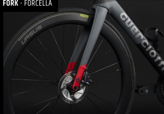
The absolute novelty of Eclipse S Disc is the fork with completely retractable cables. Designed together with the integrated handlebar, this fork gives total aerodynamics and perfect aesthetics to the bike.
