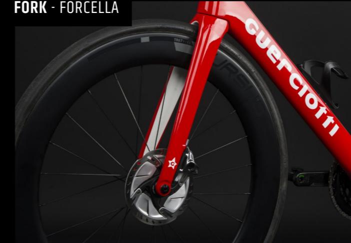
The absolute novelty of Eureka Air Disc is the fork with completely retractable cables. Designed together with the ALL IN handlebar, this fork gives total aerodynamics and perfect aesthetics to the bike.
