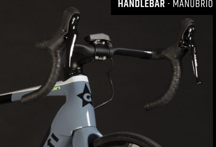
With the integral Cable System the wires are integrated within the stem and handlebar, completely hidden. This allows a substantial increase in aerodynamic, while giving you an aesthetically astonish frameset.
