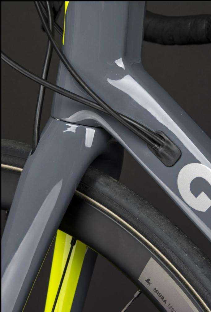
Cartesio comes with an integrated cable routing system: this make the bike beautiful like a top-class model. The predisposition of the frame for electronic groups places Cartesio a step ahead the common entry level models.
